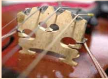
Recording string waveforms with sensors on the bridge (left) and measuring the violins' frequency response with a small hammer and laser vibrometer (right)
